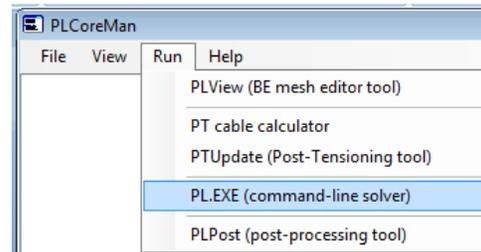
As previously stated, the PLPak creates structural analysis solutions using BE model and the Reissner Plate Equation. The main solver is the “PL.exe” command line which is retrieved from the PLCoreMan, the PL.exe creates solutions for the boundaries and supports only. In order to find solutions for any other internal points, two methods are available:
