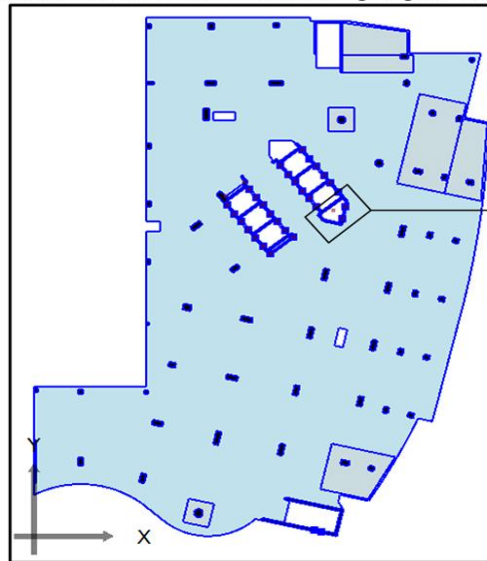
Figure 5: Another PLPAK model showing irregular shear walls
