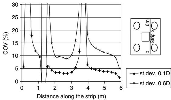
Fig. 19a. COV for  $M_{yy}$  along the second strip due to the random dislocation of pile P3—case of “ordinary” moment.
