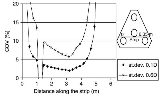
Fig. 17a. COV for  $M_{xx}$  along the strip due to the random dislocation of pile P3—case of “ordinary” moment.
