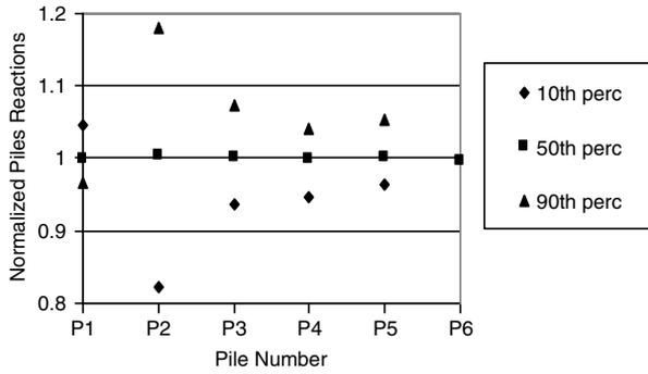
**Fig. 6.** Normalized pile reactions for different percentiles due to random dislocation of pile P4 with a standard deviation 0.6D—case of “increased” moment, 6-pile configuration.
