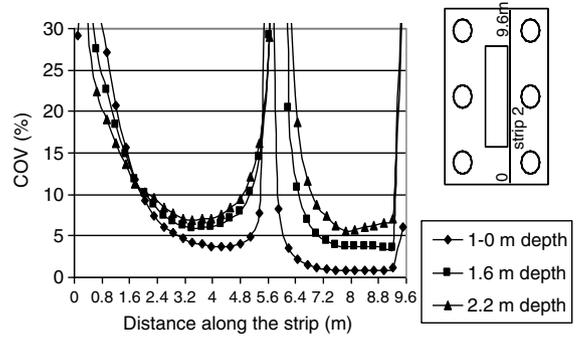
Fig. 20a. Effect of pile cap rigidity on the COV for  $M_{yy}$  along the second strip due to the random dislocation of pile P4 with a standard deviation of 0.6D—case of “increased” moment.
