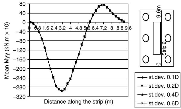
Fig. 16b. Mean  $M_{yy}$  along the second strip due to the random dislocation of pile P4—case of “increased” moment.
