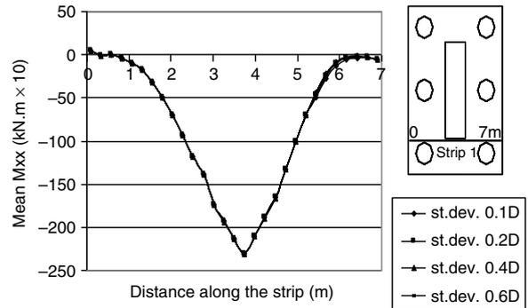
**Fig. 13b.** Mean  $M_{xx}$  along the first strip due to the random dislocation of pile P4—case of ‘‘ordinary’’ moment.
