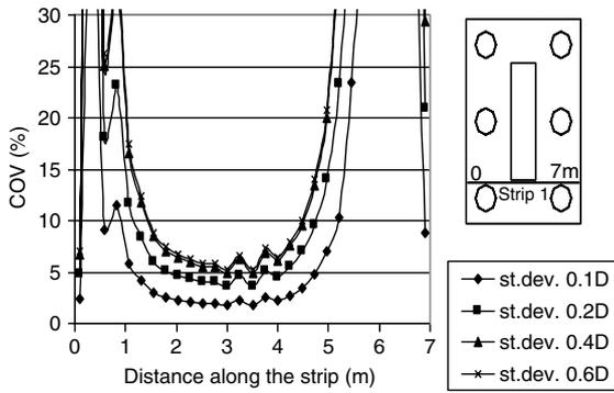
Fig. 15a. COV for  $M_{xx}$  along the first strip due to the random dislocation of pile P4—case of “increased” moment.
