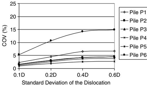
**Fig. 9b.** Effect of the standard deviation of the random dislocation on the COV for pile reactions due to the random dislocation of pile P4—case of “ordinary” moment, 6-pile configuration.
