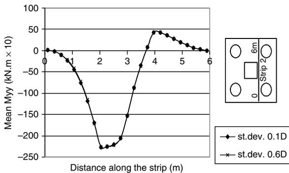
Fig. 19b. Mean  $M_{yy}$  along the second strip due to the random dislocation of pile P3—case of “ordinary” moment.
