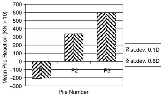
**Fig. 10a.** Mean pile reactions due to the random dislocation of pile P3 with different standard deviations—case of “ordinary” moment, 3-pile configuration.
