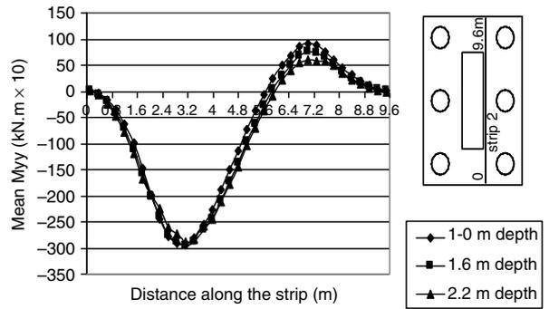
Fig. 20b. Effect of pile cap rigidity on the mean  $M_{yy}$  along the second strip due to the random dislocation of pile P4 with a standard deviation of 0.6D—case of “increased” moment.
