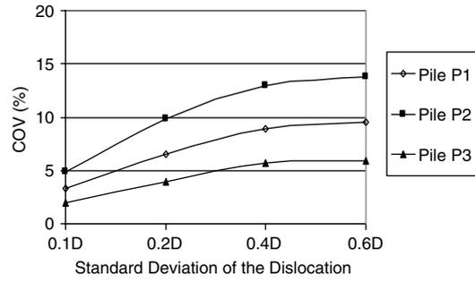
**Fig. 10c.** Effect of the standard deviation of the random dislocation on the COV for pile reactions due to the random dislocation of pile P3—case of “increased” moment, 3-pile configuration.
