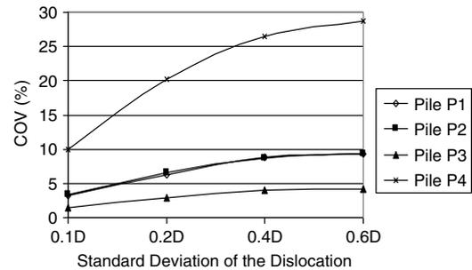
**Fig. 11c.** Effect of the standard deviation of the random dislocation on the COV for pile reactions due to the random dislocation of pile P3—case of “increased” moment, 4-pile configuration.
