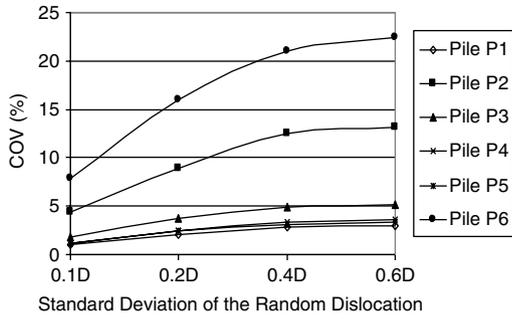
**Fig. 9a.** Effect of the standard deviation of the random dislocation on the COV for pile reactions due to the random dislocation of pile P4—case of “increased” moment, 6-pile configuration.
