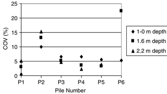
**Fig. 12.** Effect of pile cap rigidity on the COV for pile reactions due to the random dislocation of pile P4 with a standard deviation of 0.6D—case of ‘‘increased’’ moment, 6-pile configuration.
