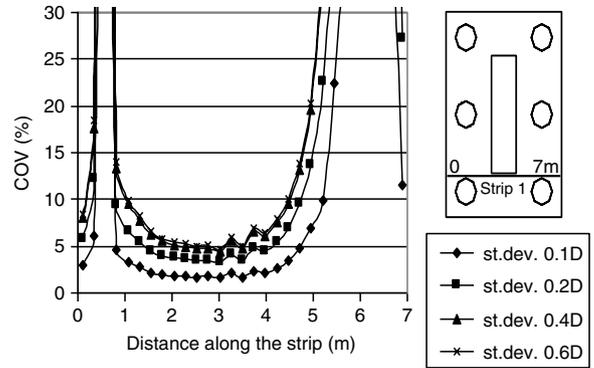
**Fig. 13a.** COV for  $M_{xx}$  along the first strip due to the random dislocation of pile P4—case of ‘‘ordinary’’ moment.
