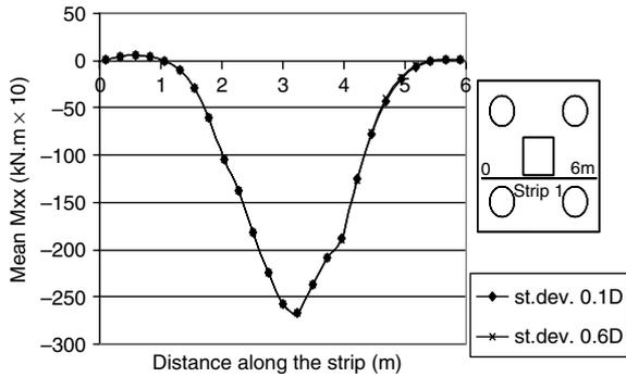
Fig. 18b. Mean  $M_{xx}$  along the first strip due to the random dislocation of pile P3—case of “ordinary” moment.
