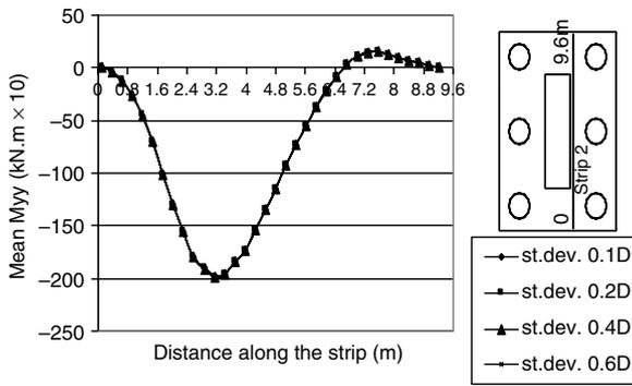
Fig. 14b. Mean  $M_{yy}$  along the second strip due to the random dislocation of pile P4—case of “ordinary” moment.
