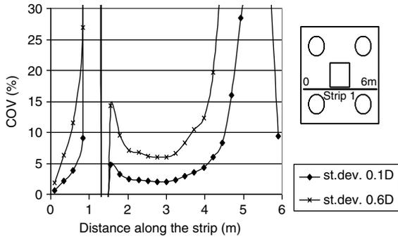
Fig. 18a. COV for  $M_{xx}$  along the first strip due to the random dislocation of pile P3—case of “ordinary” moment.
