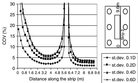
Fig. 16a. COV for  $M_{yy}$  along the second strip due to the random dislocation of pile P4—case of “increased” moment.
