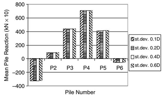
**Fig. 8b.** Mean pile reactions due to the random dislocation of pile P4 with different standard deviations—case of “increased” moment, 6-pile configuration.
