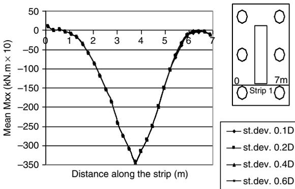
Fig. 15b. Mean  $M_{xx}$  along the first strip due to the random dislocation of pile P4—case of “increased” moment.
