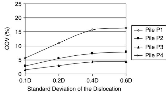
**Fig. 11b.** Effect of the standard deviation of the random dislocation on the COV for pile reactions due to the random dislocation of pile P3—case of “ordinary” moment, 4-pile configuration.
