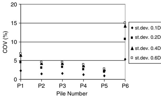
**Fig. 7a.** COV for pile reactions due to the random dislocation of pile P4 with different standard deviations—case of “ordinary” moment, 6-pile configuration.
