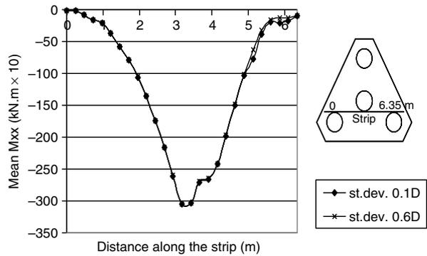
Fig. 17b. Mean  $M_{xx}$  along the strip due to the random dislocation of pile P3—case of “ordinary” moment.
