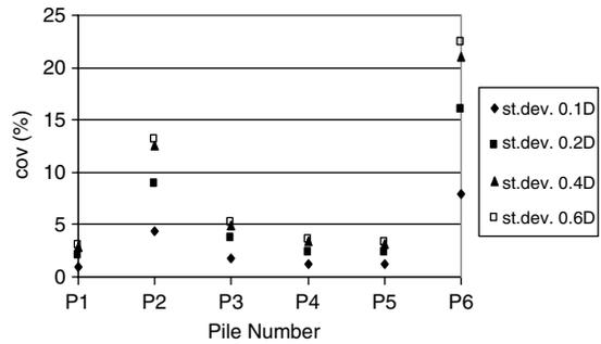
**Fig. 8a.** COV for pile reactions due to the random dislocation of pile P4 with different standard deviations—case of “increased” moment, 6-pile configuration.
