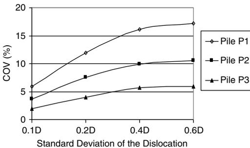
**Fig. 10b.** Effect of the standard deviation of the random dislocation on the COV for pile reactions due to the random dislocation of pile P3—case of “ordinary” moment, 3-pile configuration.
