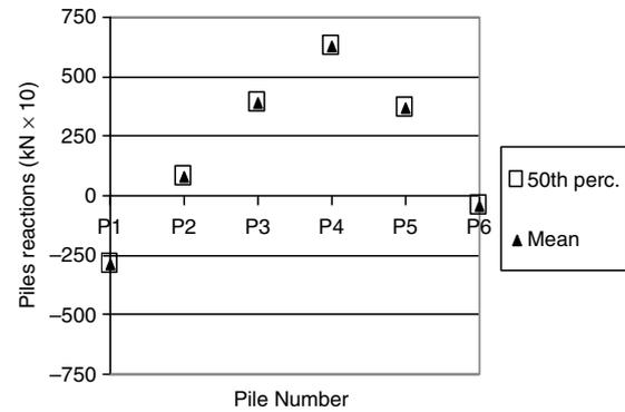
Fig. 5. The 50th percentile and the mean for pile reactions due to random dislocation of pile P4 with a standard deviation of  $0.6D$ —case of “increased” moment, 6-pile configuration.
