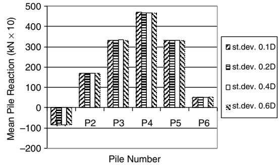
**Fig. 7b.** Mean pile reactions due to the random dislocation of pile P4 with different standard deviations—case of “ordinary” moment.
