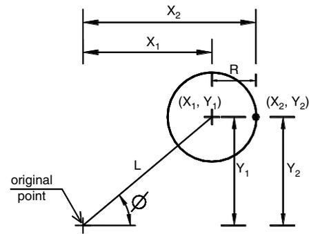
**Fig. 4.** Schematic for the random shift of pile location.
