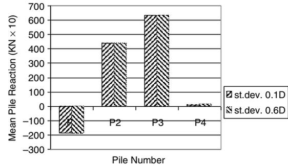
**Fig. 11a.** Mean pile reactions due to the random dislocation of pile P3 with different standard deviations—case of “ordinary” moment, 4-pile configuration.
