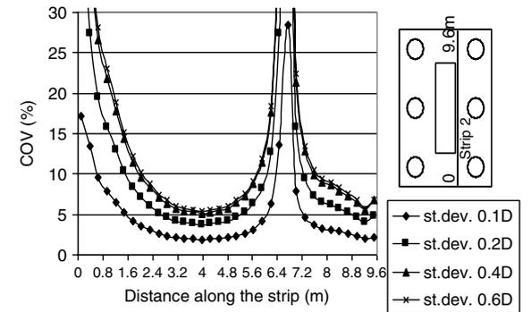
**Fig. 14a.** COV for  $M_{yy}$  along the second strip due to the random dislocation of pile P4—case of ‘‘ordinary’’ moment.
