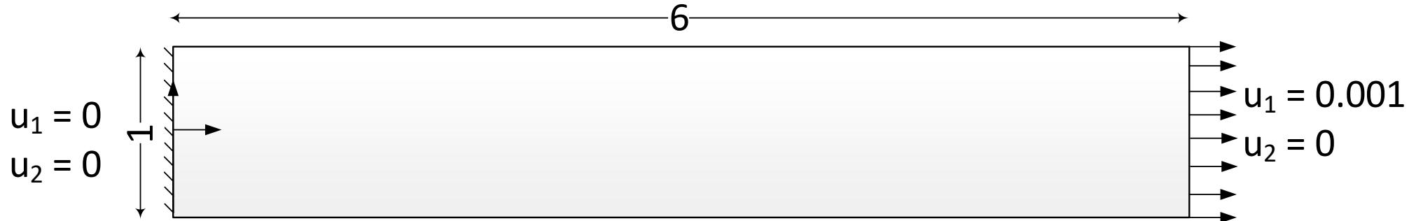
The first elasticity problem is a  $1 \times 6$  bar element subjected to 0.001 displacement at one of its ends.
